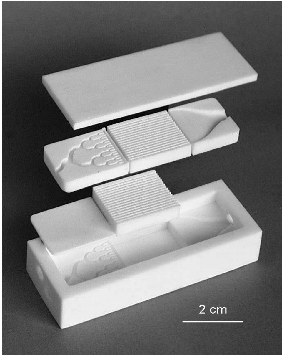
Figure 10 Modular ceramic microreactor. Individual parts are made from alumina, shaped by a RPPC. (The reactor housing has a length of 68 mm).
