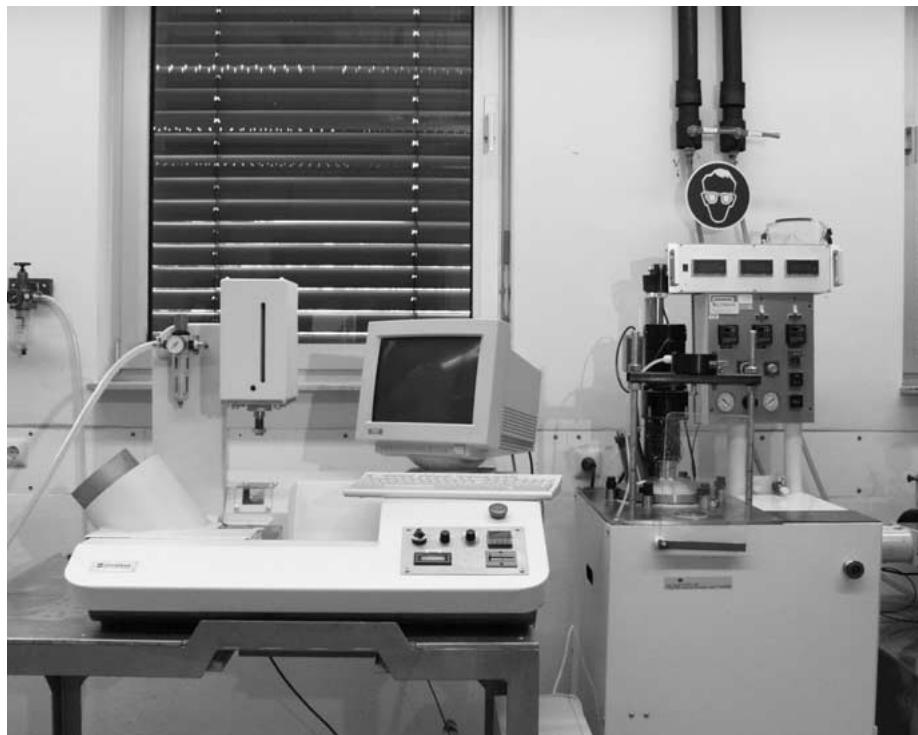
Figure 2 Low pressure injection molding machines from GOCERAM I. V. (left) and Peltsman Corp. (right).
